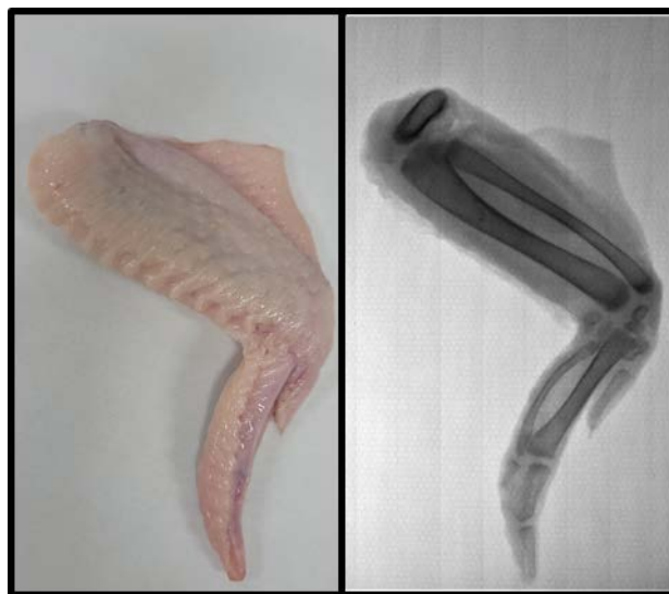
Figure 7. X-ray image of a chicken wing taken using the CNT-based stationery multi X-ray system.
