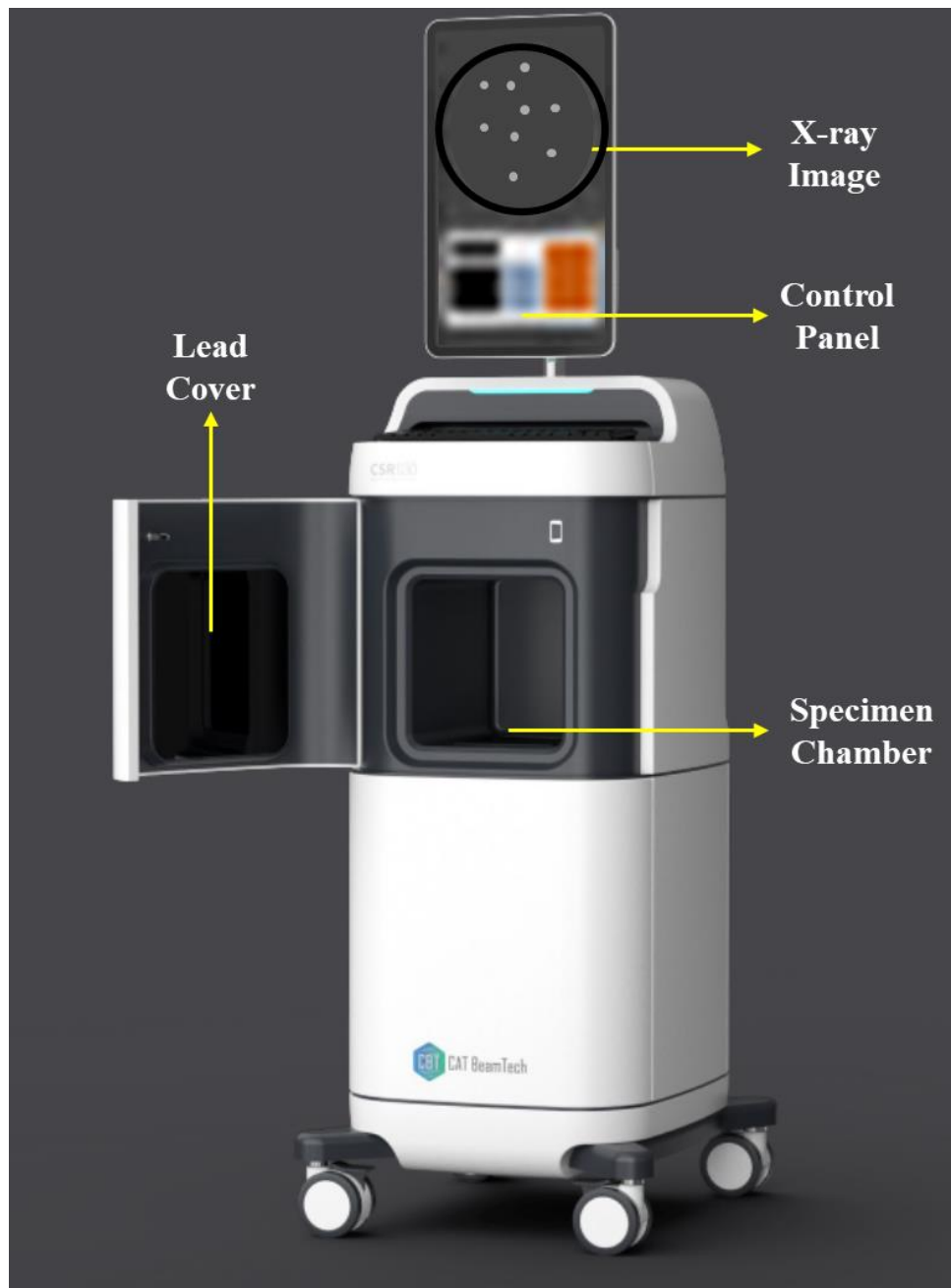
Figure 1: A 3D rendered diagram of intraoperative breast specimen system, which is being developed at CAT Beam Tech. Co., Ltd.
